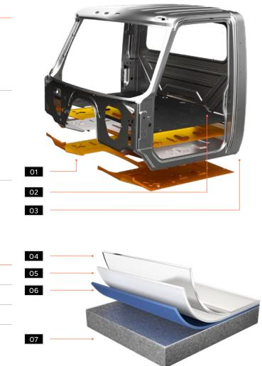
Sled Runners (day cab and sleeper) The HX Series cab variants feature high-strength steel sled runners for
