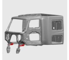
Strut Brace (sleeper only) A strut brace improves dash endurance.
