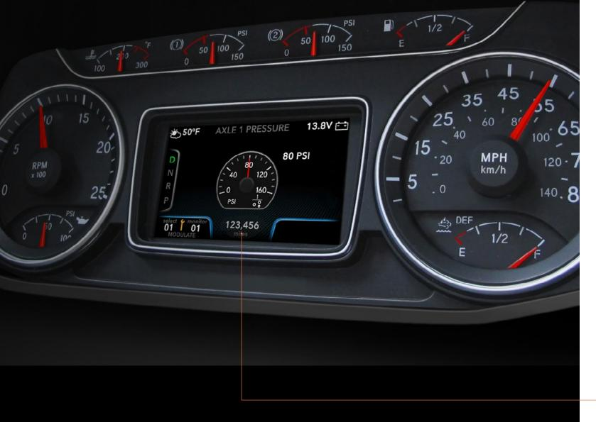
The color, illumination, legibility and even the type font and size of gauges are designed to deliver optimal viewing in varying light conditions, maximizing alertness and minimizing eye fatigue.
