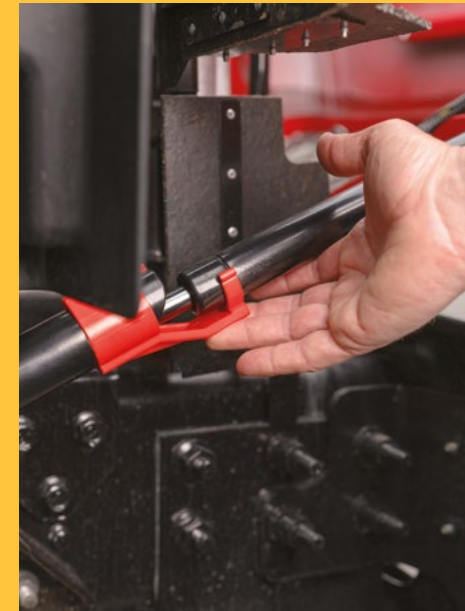
Integrated hood safety latch helps prevent the hood from blowing down on windy days.
