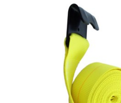
Winch Strap FLTWSF66180 Flat hook end, ratchet strap tie down, 5,400 working load, 30' length, 4" wide.
